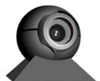
picture of the object. It is very much similar to a digital camera as it works in the same way as the digital camera with digitised images. The only difference is you cannot use Web camera without attaching it to the computer system but digital camera can be used with or without attaching it to the computer system. Web camera is specially used for video conferencing or conversation on the Internet.
