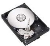
high speed, read/write heads at the end of a metal fork swing in and out to access the sectors of the disks.
